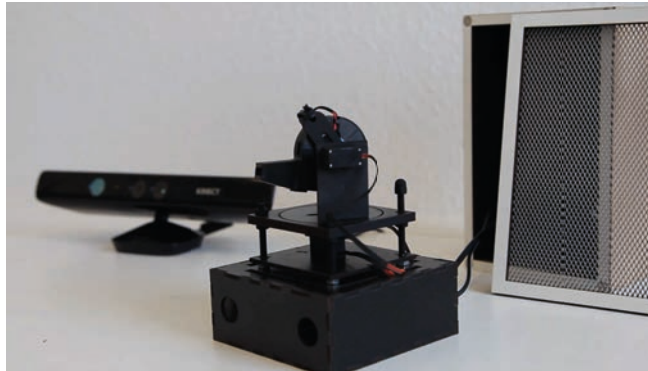
Figure 2: Two motors rotating the fan on the X- and Y axis.
